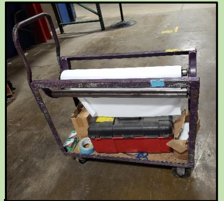
VINYL CART Used during tradeshow setup to install vinyl on Tradeshow Tables
