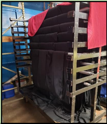
DRAPE RACK Used to transport threaded drape bars
