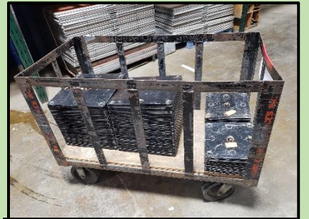
BASEPLATE CART Used to transport baseplates during tradeshow and pipe and drape installation
