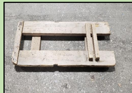
CHAIR PALLET Used to stack "Sam" style and Fruitwood / Poly chairs on for transport and storage
