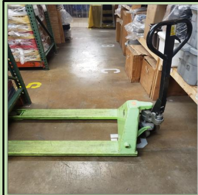
PALLET JACK Used to move pallets around warehouse or on jobsite.
