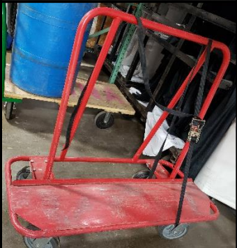
VERTICAL CARTS Used to transport items on jobsite
