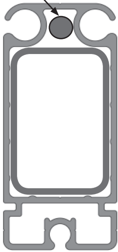
Cross sectional view of upright.
